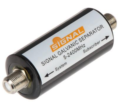
In large installations the potentials differences between particular system parts causes overvoltages during connection the devices like splitters or amplifiers, they can damage the device or cause slight electric shock. The SG-4170 is overvoltage protection of the receivers operating in terrestrial TV full band. It is used for example to protection of: TV receivers, HiFi sets, amplifiers.
