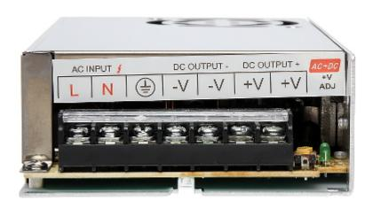
L - Live wire (230V) N - Neutral wire GND - Grounding -V - DC "-" output +V - DC "+" output ADJ - Output voltage adjustment
