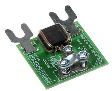
The SA/I-III-DIPOL antenna impedance transformer matches the antenna impedance to the impedance of coaxial cable.
