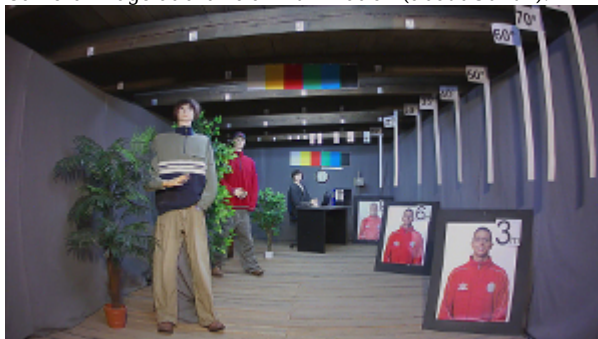
Camera image at artificial illumination (about 30Lux):
