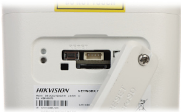
Memory card slot and "Reset" button:
