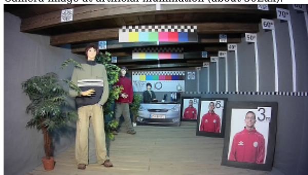
Camera image at artificial illumination (about 30Lux):
