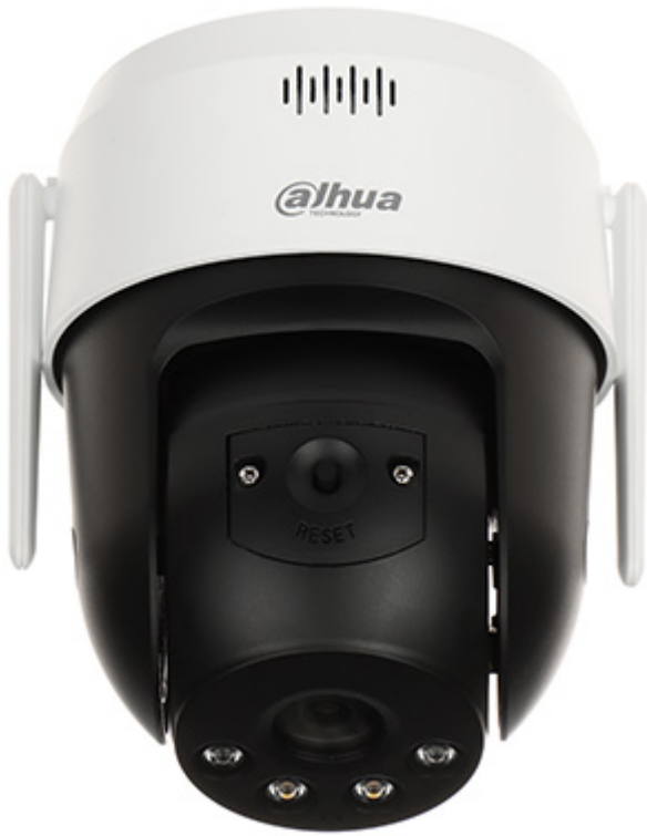
Memory card slot and "Reset" button:
