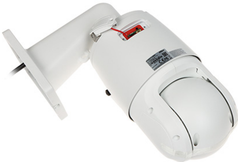
Memory card slot and "Reset" button:
