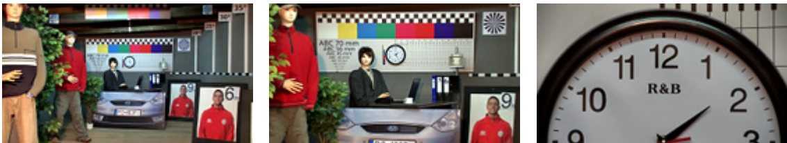
Camera image at night conditions with internal built-in IR illuminator on:
