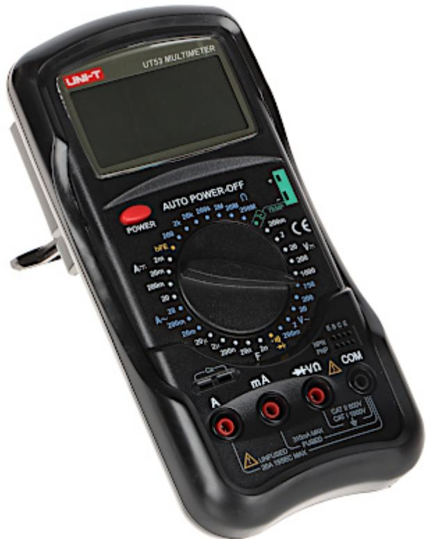
The UT-53 is a universal digital meter used to measure: voltage, current, resistance, capacitance, hFE, temperature and checking the correct operation of diodes.
