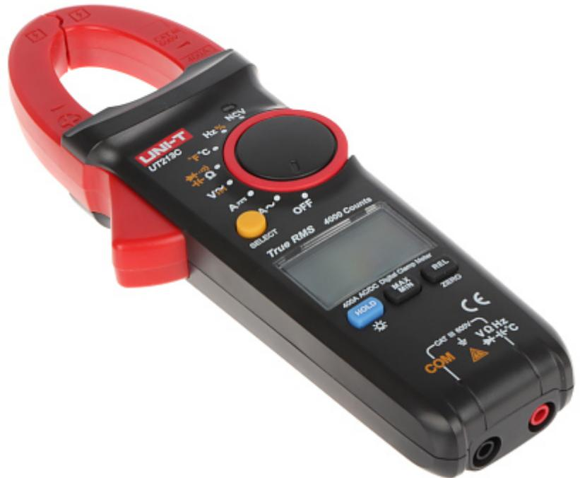
The UT-213C is a universal digital meter equipped with clamps enabling the measurement of high currents. The device measures: voltage, current, frequency, resistance, capacity and temperature. In addition, the meter has an electric field detection function (NCV).
