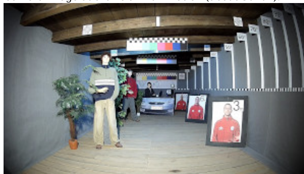
Camera image at artificial illumination (about 30Lux):
