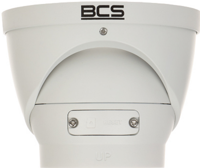
Memory card slot and "Reset" button:
