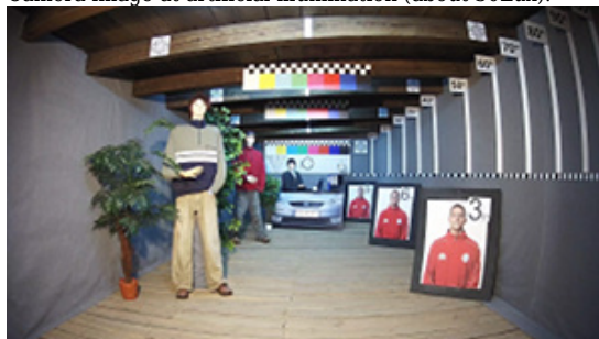
Camera image at artificial illumination (about 30Lux):
