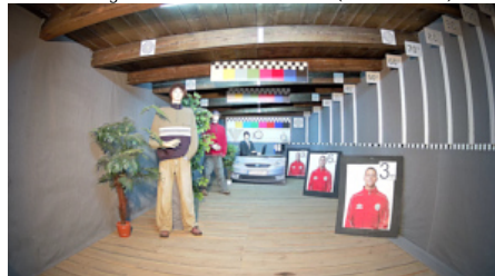
Camera image at artificial illumination (about 30Lux):
