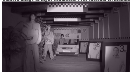
Camera image at night conditions with external IR illuminator on:
