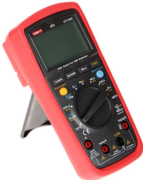
The UT-139C is a universal digital meter used to measure: voltage, current, resistance, capacity, frequency, temperature and checking the correct operation of diodes. EF function - enables non-contact voltage detection eg in wires, in the range of 50V ... 400V.
