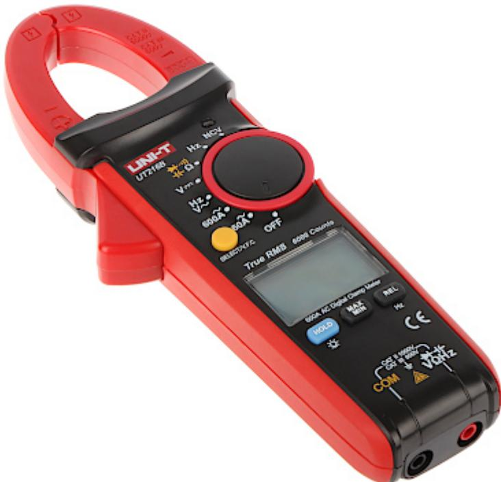
The UT-216B is a universal digital meter equipped with clamps enabling the measurement of high currents. The device measures: voltage, current, frequency, resistance and capacity. In addition, the meter has an electric field detection function (NCV).
