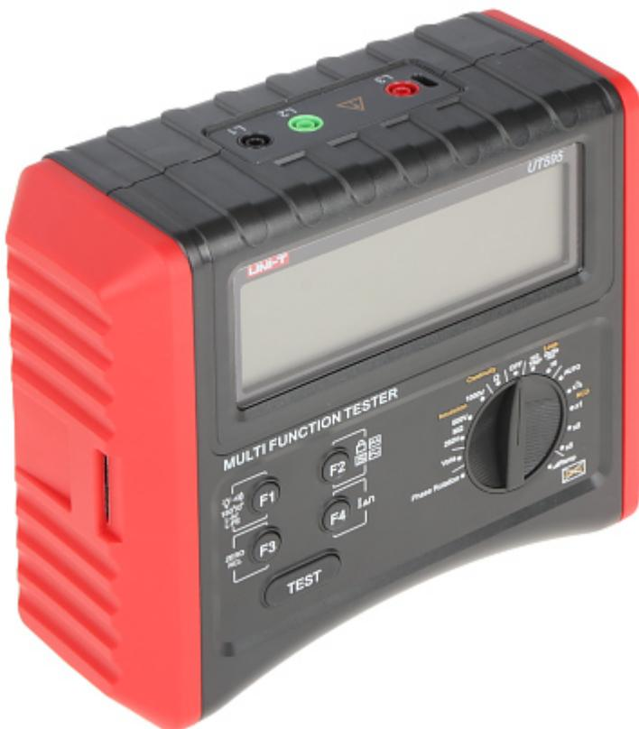
The UT-595 is a multifunction meter for measurements in electrical installations, dedicated to electricians. The device is also a comprehensive tester for the safety of electrical installations. The UT-595 allows you to measure insulation resistance, short circuit loop impedance with/without RCD tripping, line impedance, continuity of protective and equalizing conductors, test of trip current and RCD tripping time, AC voltage value, and the phase sequence display.
