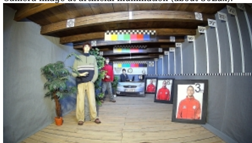
Camera image at artificial illumination (about 30Lux):
