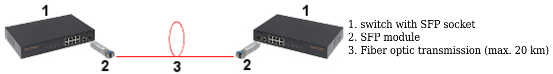
Connection diagram:
