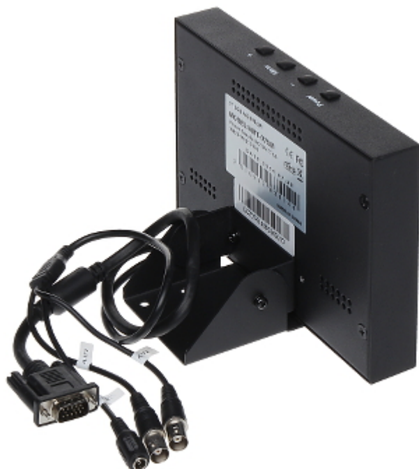
Bracket enables to mount to flat, sloping or horizontal surfaces:
