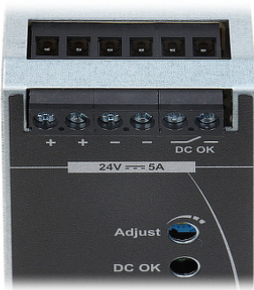
Rear panel (DIN rail installation):
