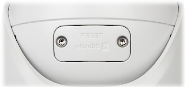
Memory card slot and "Reset" button:
