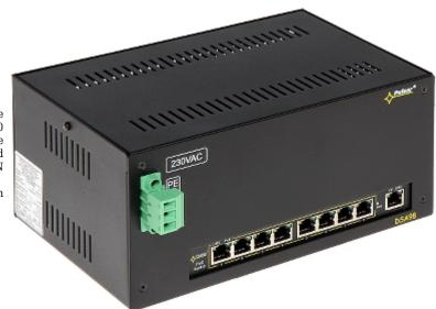
The DSA-98 PoE Switch is an industrial type device enabling fluent network transmission at rates 10 / 100 Mbps. PoE powering possibility, compatible with the 802.3af standard makes the device more universal and easier to install. DSA-98 is designed to mount on the DIN 35 mm rail.
