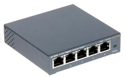
The device is widely used in small computer networks, neighborhood networks. It has built-in the Auto MDI/MDIX function, which does not bother the installer about the problem of straightforward or crossover cables.
