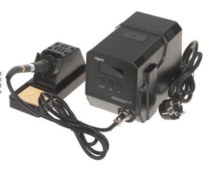
The PR-ZD-8936 soldering station with the power of 48 W has adjustable tip temperature in the range of 160 °C ... 480 °C. The soldering iron has a standard conical tip, but the offer also includes other types of tips dedicated to work with this model of soldering station.
