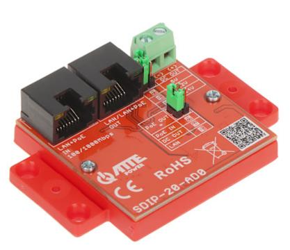
The SDIP-20-AD0 adapter is designed to power additional devices via a PoE line or reduce the PoE voltage present in the RJ45 plug with a bandwidth of 10/100/1000 Mbps. Appropriate jumper combinations allow to select the appropriate PoE power supply configuration at the output as well as the output voltage level from the converter.
