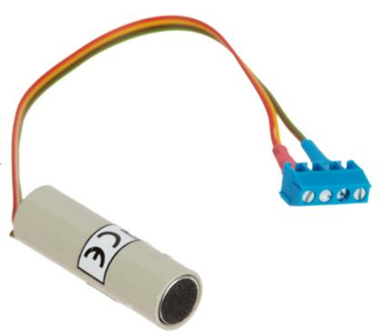
MP-6/D is designed for listening to the outside sounds. The device has a differential (symmetrical) output, which allows to signal transmission via twisted-pair cable and also an asymmetrical output, to signal transmission via coaxial cable. The advantage of differential transmission of sound via UTP cable is elimination the interferences and hum noise generated at the cable. The asymmetrical signal can be obtained by connection between (-) power signal and one of the symmetrical output.
