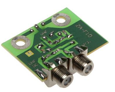
The multiplexer is designed for installation inside VHF/FM antenna boxes. The device has built-in impedance transformer for mounting directly in the VHF/FM antenna boxes.
