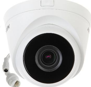
IP camera with efficient H.264 image compression algorithm for clear and smooth video streaming at maximal resolution of 1080p. Due to above it is perfect solution for surveillance systems requiring persons or vehicles recognition. The used motozoom lens with 2.8 ... 12 mm focal length allows to remote view angle adjustment.
