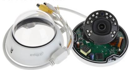
Micro SD card slot is located inside the camera:
