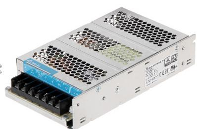
Power adapter with two pairs of output terminals. Attention! If the power adaptor is using for continuous work (24H) the rated current of the adaptor should be less than 80% of the maximal current.
