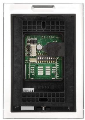
On the body, under the cover there are placed configuration switches:
