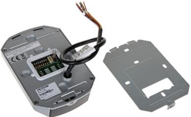
On the body, under the cover there are placed configuration switches:
