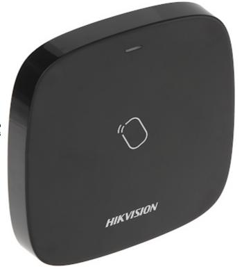
Wireless external card and keyfob reader. The device is designed to work with the Hikvision and Pyronix wireless access control systems operating in the  $868~\mathrm{MHz}$  band.
