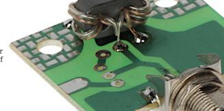
The SA/I-V/F-DIPOL antenna impedance transformer matches the antenna impedance to the impedance of coaxial cable.
