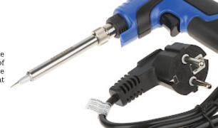
The LUT-0071 pistol soldering iron when connected to the power source heats up and maintains the temperature of the tip at about 200 °C. Pressing the button increases the power consumption to 130 W, thus allowing the tip to heat up to a temperature of up to 450 °C.
