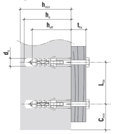
$$\label{eq:hole_drill} \begin{split} & \text{Hole/drill diameter } [d_o] \text{ - } 10 \text{ mm} \\ & \text{Min. substrate thickness } [h_{\text{min}}] \text{ - } 90 \text{ mm} \\ & \text{Drilled hole depth } [h_o] \text{ - } 70 \text{ mm} \\ & \text{Anchorage depth } [h_{\text{eff}}] \text{ - } 60 \text{ mm} \end{split}$$
