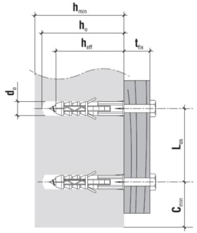
$$\label{eq:hole_drill} \begin{split} & Hole/drill\ diameter\ [d_0] - 12\ mm \\ & Min.\ substrate\ thickness\ [h_{min}] - 120\ mm \\ & Drilled\ hole\ depth\ [h_0] - 90\ mm \end{split}$$
