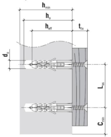
$$\begin{split} & \text{Hole/drill diameter } [d_o] \text{ - 8 mm} \\ & \text{Min. substrate thickness } [h_{\text{min}}] \text{ - 75 mm} \\ & \text{Drilled hole depth } [h_o] \text{ - 60 mm} \\ & \text{Anchorage depth } [h_{\text{eff}}] \text{ - 50 mm} \\ & \text{Max. usable length } [t_{\text{fix}}] \text{ - 30 mm} \end{split}$$
