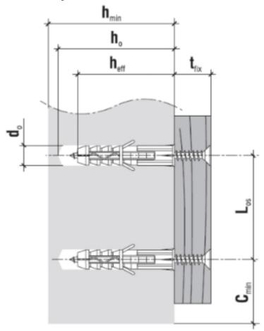
$$\label{eq:hole_def} \begin{split} & Hole/drill \; diameter \; [d_o] - 10 \; mm \\ & Min. \; substrate \; thickness \; [h_{min}] - 75 \; mm \\ & Drilled \; hole \; depth \; [h_o] - 60 \; mm \\ & Anchorage \; depth \; [h_{eff}] - 50 \; mm \end{split}$$
