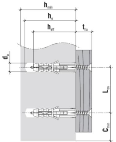
$\begin{array}{l} Hole/drill \ diameter \ [d_{o}] \ - \ 10 \ mm \\ Min. \ substrate \ thickness \ [h_{min}] \ - \ 90 \ mm \\ Drilled \ hole \ depth \ [h_{o}] \ - \ 70 \ mm \\ Anchorage \ depth \ [h_{eff}] \ - \ 60 \ mm \\ Max. \ usable \ length \ [t_{fix}] \ - \ 40 \ mm \\ \end{array}$
