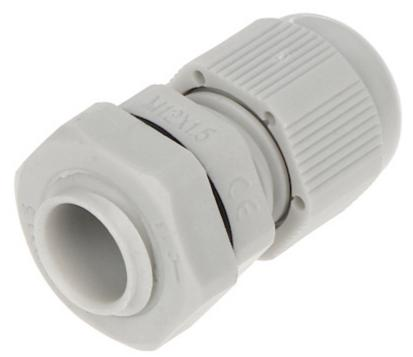
The D/M-12X1.5 cable gland is used to lead cables into an enclosure. A gland protects a cable from being cut with sharp boards of enclosure hole. Moreover it protects devices inside the enclosure from the effects of adverse external factors.
