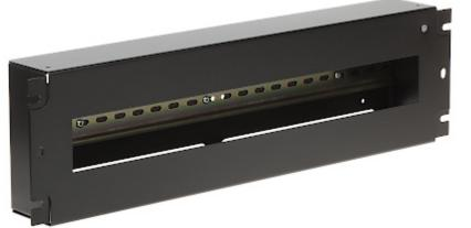
The enclosure with a DIN rail for RACK cabinets is intended for mounting equipment located inside DIN enclosures, for RACK 19" cabinets. The enclosure features a DIN rail, length: 24x1S. The height of the mounted module cannot exceed 160 mm.
