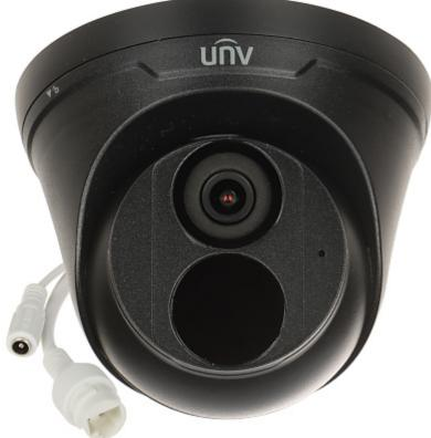
IP camera with efficient Ultra 265 image compression algorithm for clear and smooth video streaming at maximal resolution of 4 Mpx.
