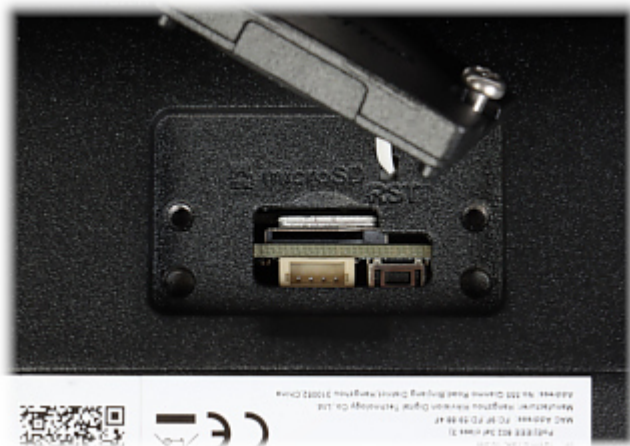
Memory card slot and "Reset" button:
