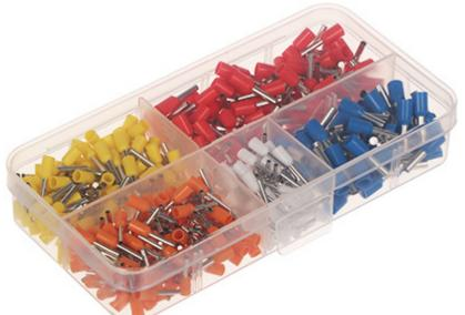
Set of cable ferrules from  $0.5~\text{mm}^2$  to  $2.5~\text{mm}^2$  with organizer. Cable ferrules are designed for clamping on the stranded wires to keep all loose cable wires together and reduce the risk of a short circuit.
