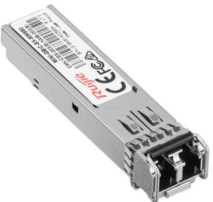
Mini-GBIC (Mini - Gigabit Interface Converter) optical modules complying with SFP (Small Form-factor Pluggable) agreement are popular and flexible way of optical telecommunication links, like 1000Mbit/s Ethernet, ATM, PDH/SDH as well as data communication with Fiber Channel HDDs or HDD arrays.
