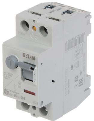
Residual current circuit breaker with rated sensitivity of I $\Delta$ n = 30mA, AC type. The HNC-25/2/003 circuit breaker is compatible to DIN TS-35 rail mounting system.
